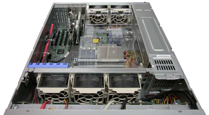
Inside view with 1x Intel Xeon CPU (passive cooled)
